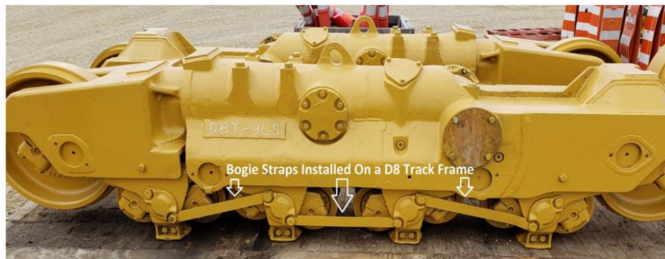
Bogie straps installed on a D8 track frame
