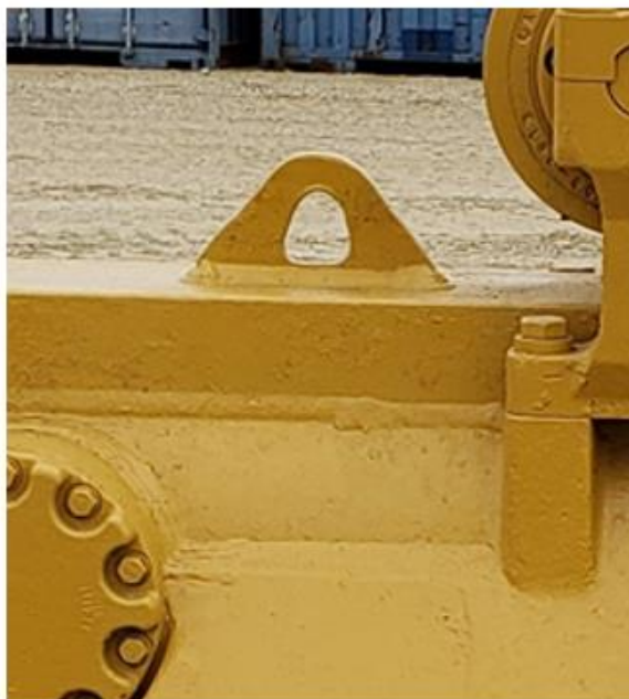
Example of a good lifting lug.
